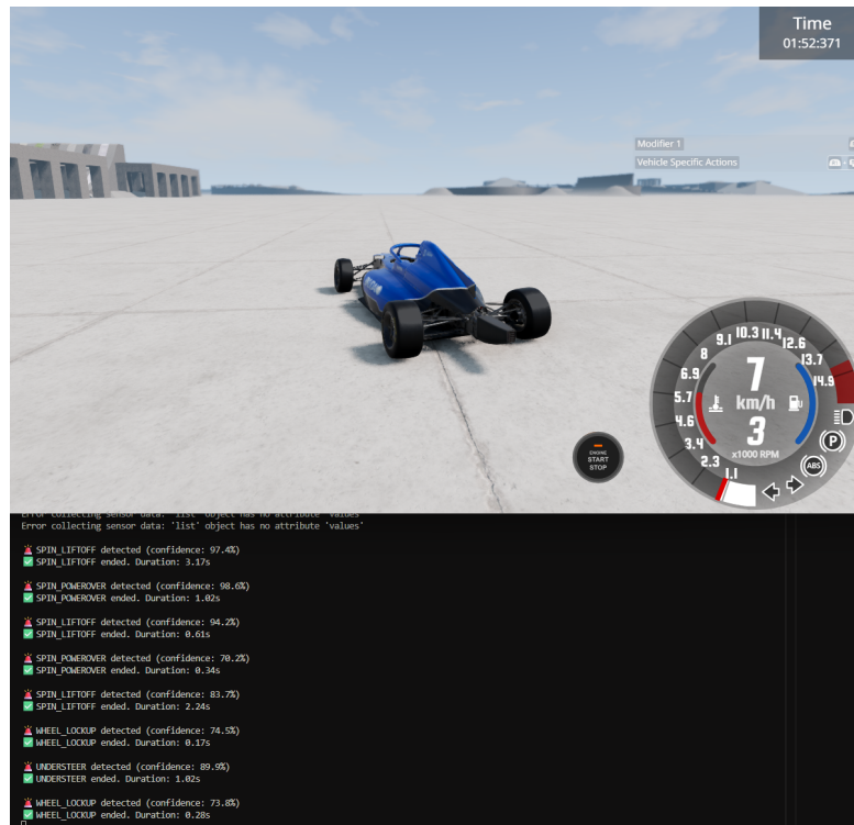
Figure 3.3: Screenshot of the live monitoring output during a test run. Detected events are printed with their predicted types and confidence scores.
